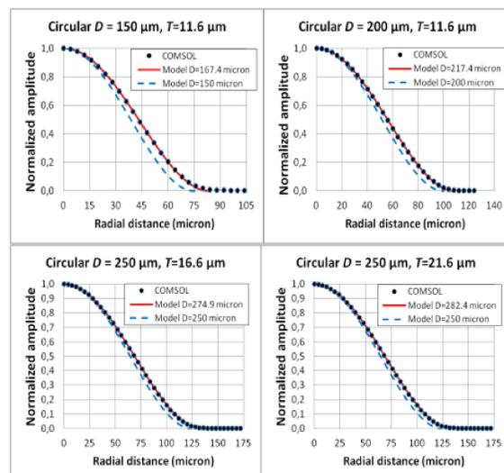
Resonant amplitude in air for circular MEMS, simulated in COMSOL (dot) and modeled analytically either using for the radial distance the diameter of the diaphragm,  $D$  (dashed), or  $D_{\text{eff}} = D + 1.5T$  (solid line), where  $T$  is the diaphragm's thickness.
