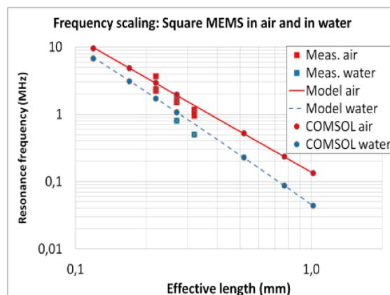
Resonance frequencies versus effective length for  $T_{\text{Si}} = 10 \mu\text{m}$  clamped square MEMS, simulated (dots), modeled (lines) and measured with a Laser Doppler Vibrometer (squares).
