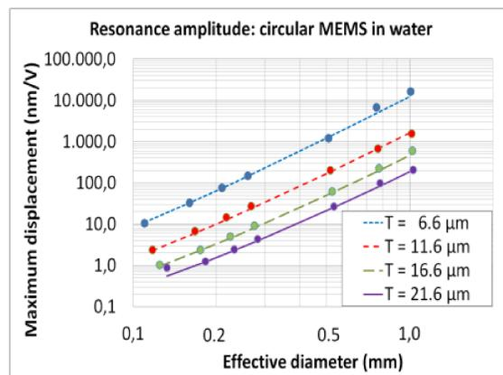
Resonance amplitude versus effective diameter for circular MEMS, simulated (dots) and modeled (lines).
