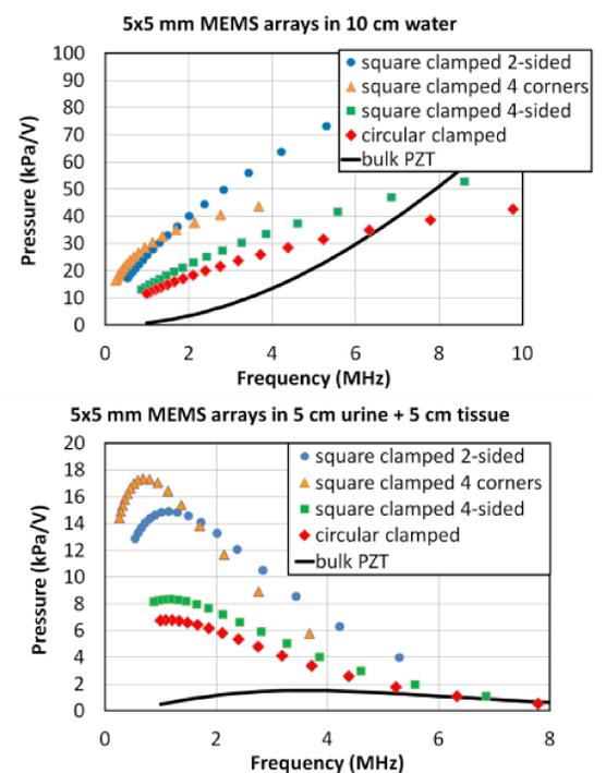
Models for the pressure generated by four types of  $5 \times 5 \text{ mm}^2$  MEMS arrays (symbols) with a  $5 \times 5 \text{ mm}^2$  bulk PZT5H transducer as a reference (line).
